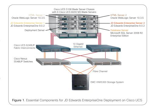
bring a high-bandwidth, low-latency, 10-Gbps unified fabric to each server that carries IP, storage, and management traffic over a single set of cables. The system represents a radical simplification compared to traditional architectures, resulting in lower capital expenditures and operating costs.
