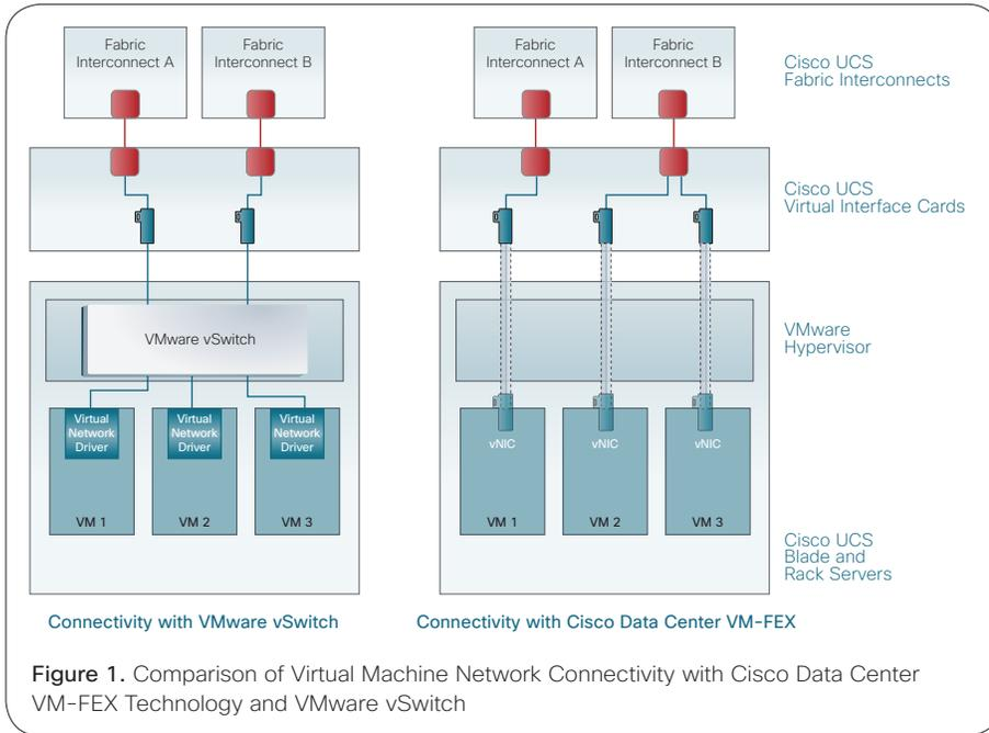
Figure 1. Comparison of Virtual Machine Network Connectivity with Cisco Data Center VM-FEX Technology and VMware vSwitch
