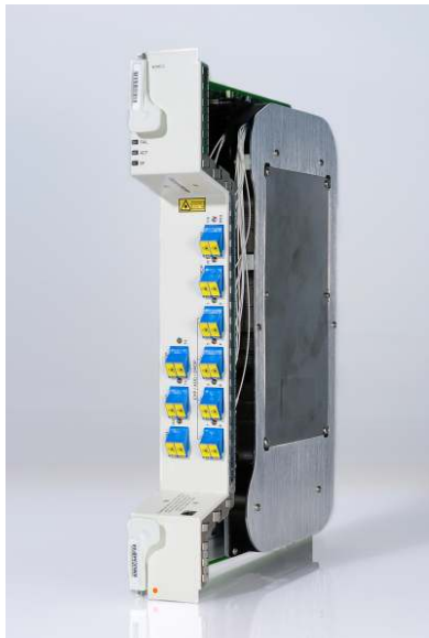
Figure 1. 80-Channel Wavelength Cross-Connect Card with Integrated Optical Channel Monitor
