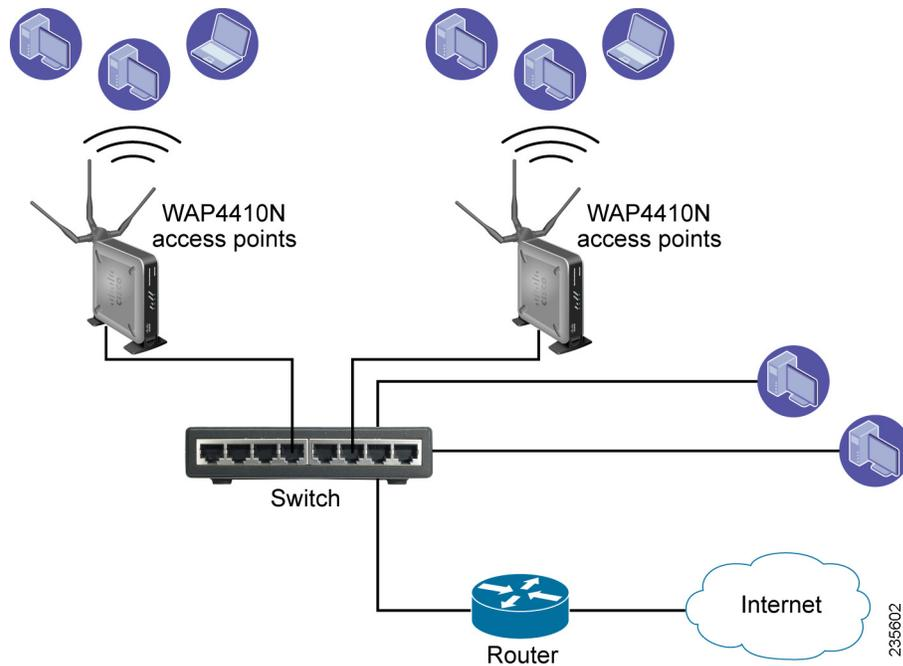
In this illustration, the switch connects to a router that connects to the Internet. The network provides connectivity among wireless network devices and computers that have a wired connection to the switch. The wireless access points connect to a Cisco switch that provides them with power. Each access point connects multiple wireless devices to the network.
