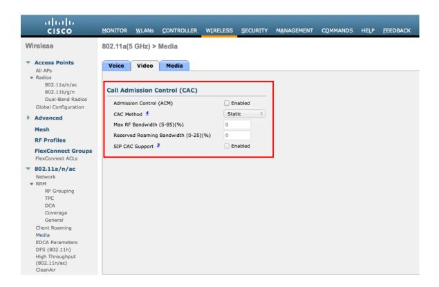
If Call Admission Control for voice is enabled, then the following configuration should be enabled, which can be displayed in the **show run-config**.
