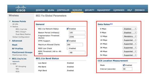
If using 2.4 GHz, ensure the 802.11b/g network status and 802.11g is enabled.
