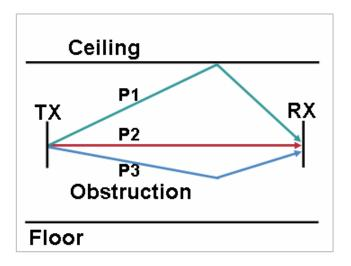
Use of Orthogonal Frequency Division Multiplexing (OFDM), which is used by 802.11a and 802.11g, can help to reduce issues seen in high multipath environments.
