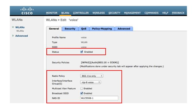
In order to utilize CCKM, enable WPA2 policy with AES encryption and 802.1x + CCKM for authenticated key management type when the Cisco Unified Wireless IP Phone 7921G is running firmware version 1.3(4) or later in order to enable fast secure roaming.
