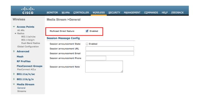
After **Multicast Direct feature** is enabled, then there will be an option to enable **Multicast Direct** in the QoS menu of the WLAN configuration.
