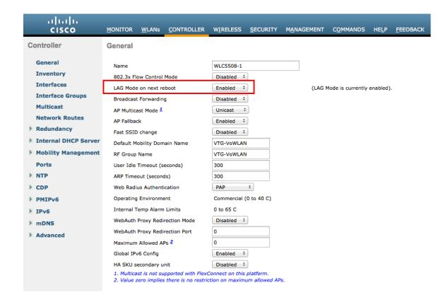
If utilizing multicast, then Enable Global Multicast Mode and Enable IGMP Snooping should be enabled.
