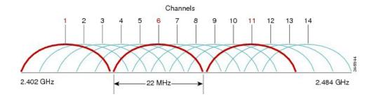
Non-overlapping channels must be used and allow at least 20 percent overlap with adjacent channels when deploying the Cisco Unified Wireless IP Phone 7921G in the 802.11b/g/n environment, which allows for seamless roaming.
