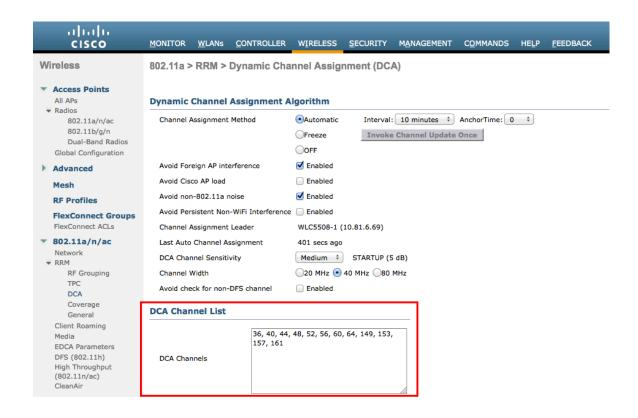
If using 2.4 GHz, only channels 1, 6, and 11 should be enabled in the DCA list.
