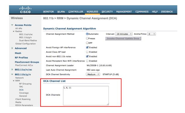
Individual access points can be configured to override the global setting to use dynamic channel and transmit power assignment for either 5 or 2.4 GHz depending on which frequency band is to be utilized.
