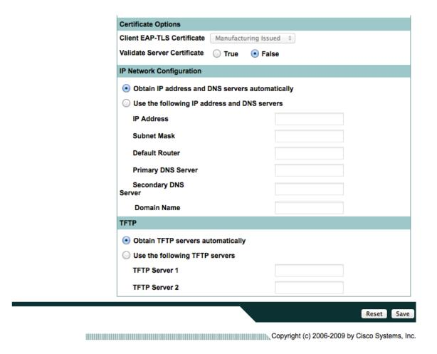
**Note:** If the TFTP IP is changed which is not included in the current Certificate Trust List (CTL) file, then TFTP will fail and may prevent the phone from registering successfully to the Cisco Unified Communications Manager. The CTL file will need to be erased manually in the Security Configuration menu from the Cisco Unified Wireless IP Phone 7921G.
