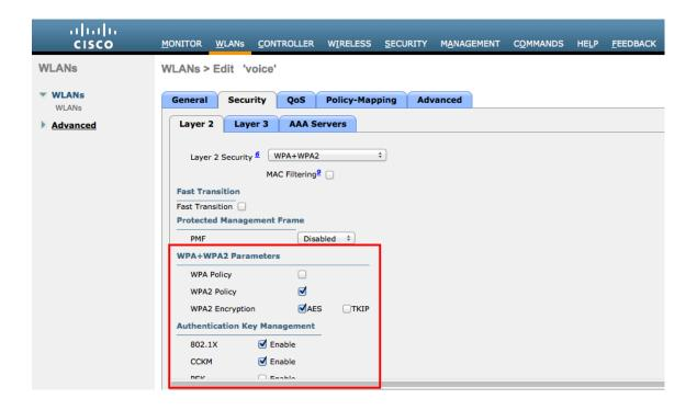
If the Cisco Unified Wireless IP Phone 7921G is running firmware version 1.3(3) or earlier, then enable WPA policy with TKIP encryption and 802.1x + CCKM for authenticated key management type in order to enable fast secure roaming.
