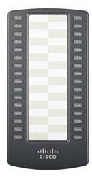
The Cisco SPA500S attendant console attaches to a Cisco SPA500 Series IP phone to provide additional feature buttons. Up to two 32-button units can be attached to a phone to provide a total of 64 feature buttons.
