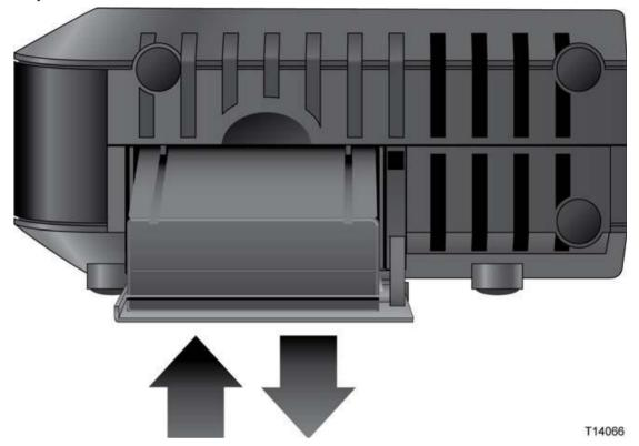
5 Close the battery compartment door. The battery lock will automatically reengage.
