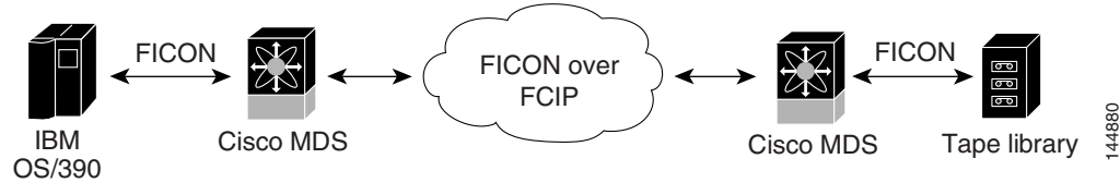
Figure 28-20 Host Directly Accessing IBM/STK (StorageTek) Library
