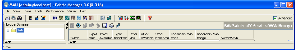
Figure 66-16 Setting secondary MAC addresses
