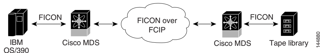
Figure 28-5 Host Directly Accessing IBM/STK (StorageTek) Library
