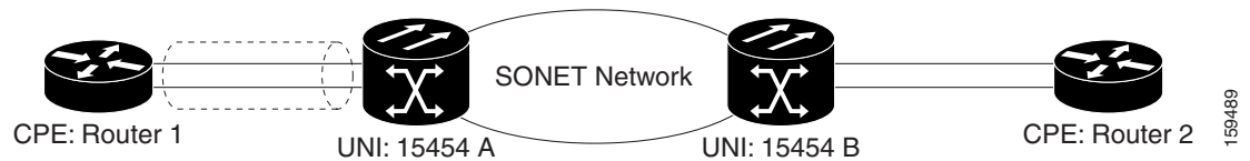
Figure 34-3 LACP Termination Mode Example
