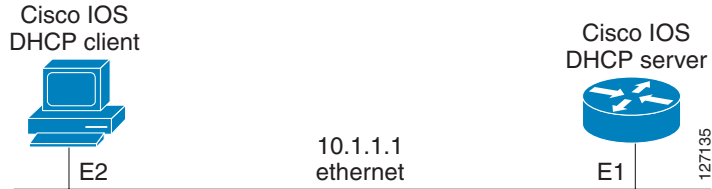
Figure 2 Topology Showing DHCP Client with Ethernet Interface
