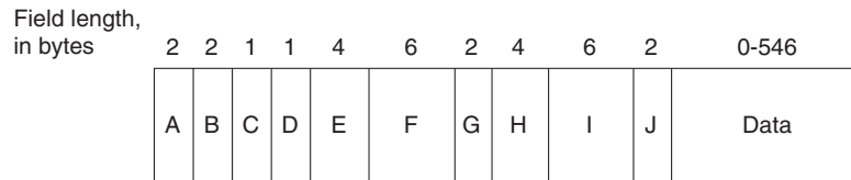
Figure 14-1 The IDP Packet Format
