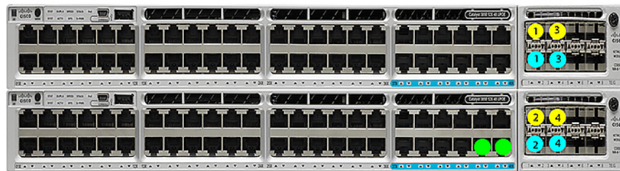
Dual 10/25GE ToR Switches (standalone or stacked)
