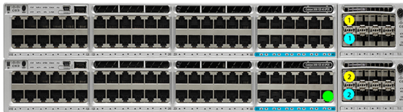
Dual 10/25GE ToR Switches (standalone or stacked)
