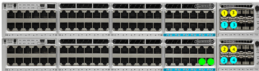
Dual 10/25GE ToR Switches (standalone or stacked)
