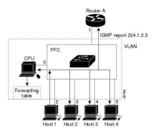
Router A sends a general query to the controller, which forwards the query to ports 2 through 5, all of which are members of the same VLAN. Host 1 wants to join multicast group 224.1.2.3 and multicasts an IGMP membership report (IGMP join message) to the group. The controller CPU uses the information in the IGMP report to set up a forwarding-table entry that includes the port numbers connected to Host 1 and to the router.
