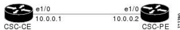
Figure 22: Configuration for Peering with Directly Connected Interfaces Between CSC-PE and CSC-CE Routers
