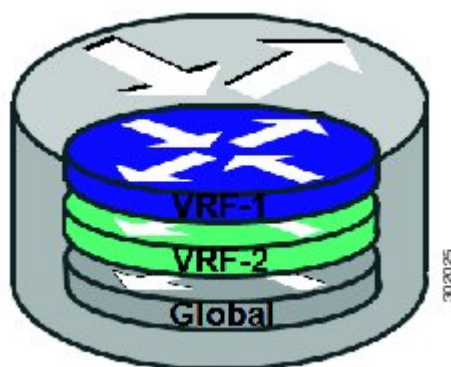
Figure 33: Device Level Virtualization
