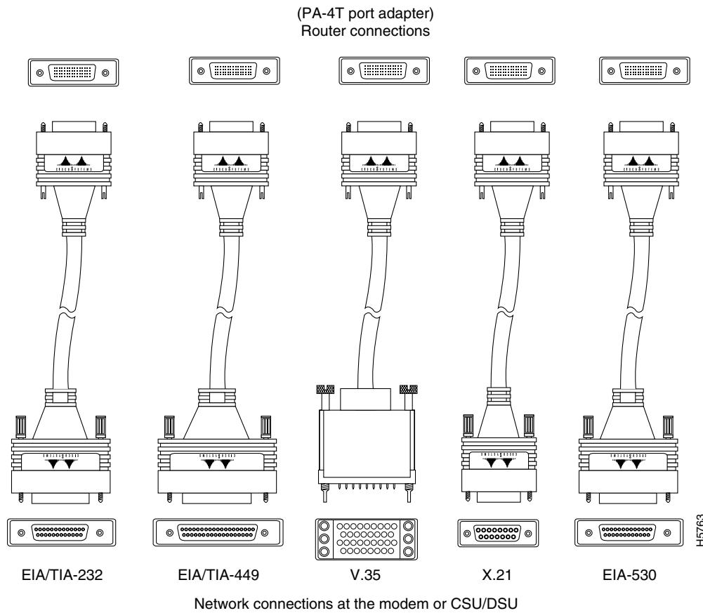
Metric (M3) thumbscrews are included with each port adapter cable to allow connections to devices that use metric hardware. Because the 4T port adapter uses a special, high-density port that requires special adapter cables for each electrical interface type, we recommend that you obtain serial interface cables from the factory.
