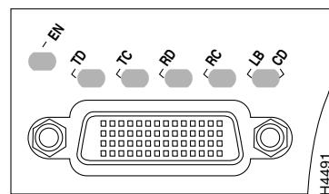
The green enabled LED on the port adapter indicates that the motherboard is enabled and receiving power, and that the port adapter is ready for operation.
