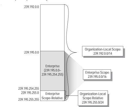
Figure 13 Correct Placement of the Enterprise Scope Relative Range
