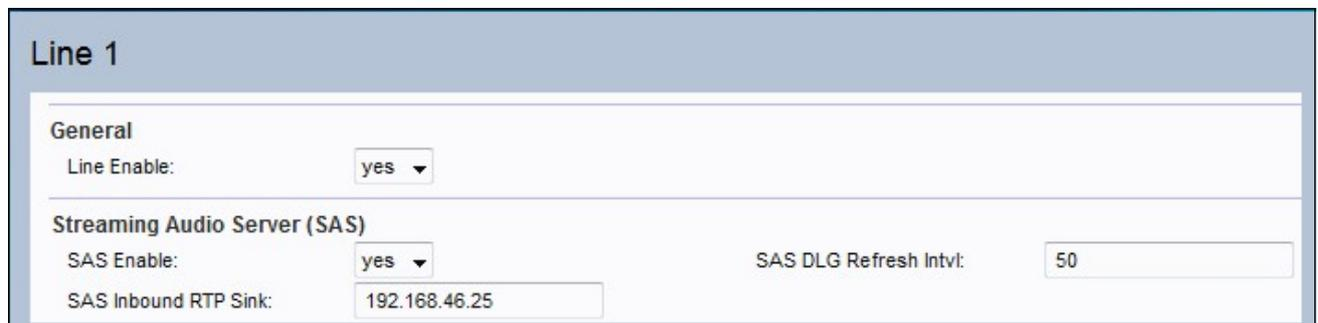
The screenshot shows the configuration page for Line 1. It has a header 'Line 1' and a 'General' section with 'Line Enable' set to 'yes'. Below that is the 'Streaming Audio Server (SAS)' section, which includes 'SAS Enable' set to 'yes', 'SAS DLG Refresh Intvl' set to '50', and 'SAS Inbound RTP Sink' set to '192.168.46.25'.
