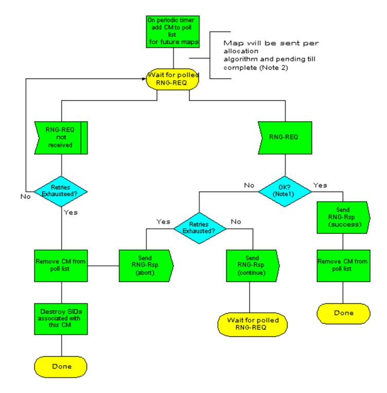
Note 1: Measures ranging request is within the tolerance limits of the CMTS for power and tra equalisation (if supported)
