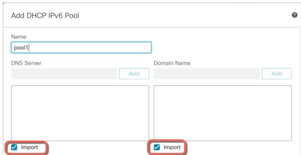
The screenshot shows the 'Add DHCP IPv6 Pool' configuration page. The 'Name' field contains 'pool1'. The 'DNS Server' and 'Domain Name' fields are empty, each with a blue 'Add' button next to it. Below the input fields are two empty boxes, each with an 'Import' checkbox that is now checked and highlighted with a red box.
