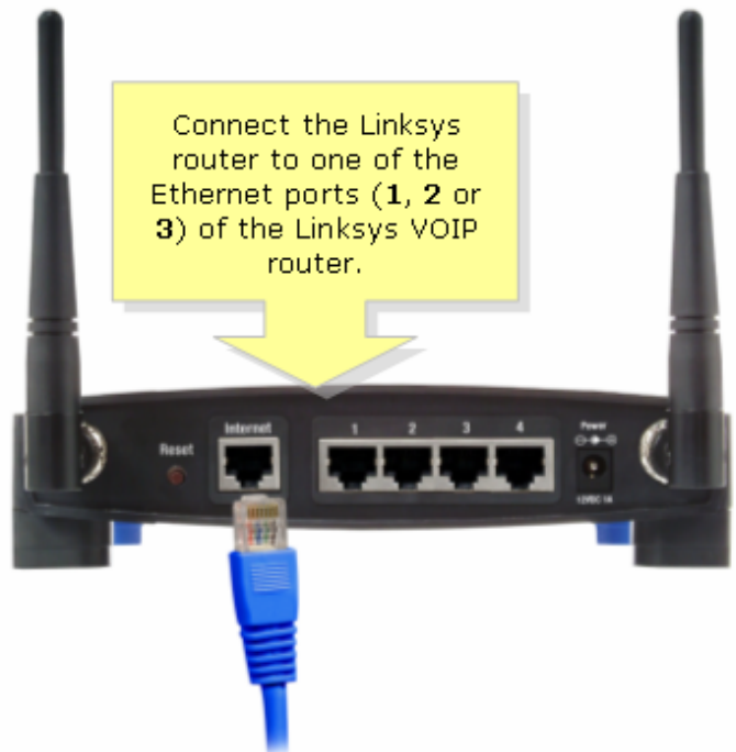
Second Router (Linksys router which will be connected to the Linksys VOIP router)
