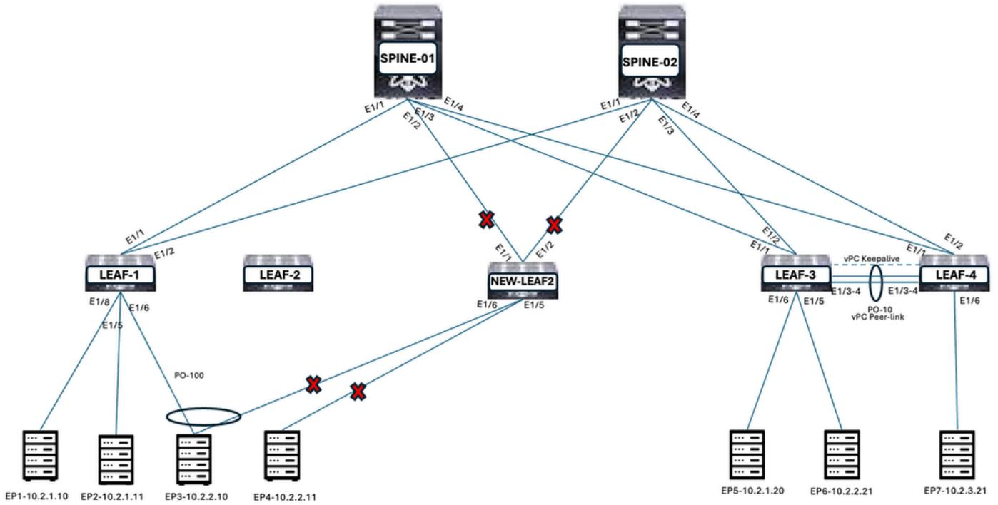
**步骤6.在NEW-LEAF2上取消关闭上行链路端口和孤立端口**
