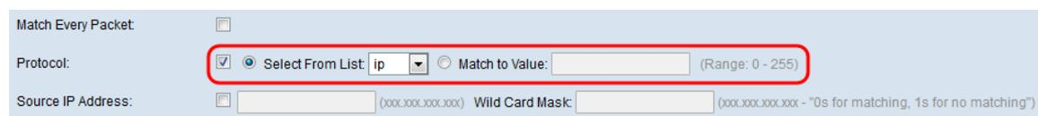
The screenshot shows the configuration page for an ACL rule. The 'Protocol' checkbox is checked and highlighted with a red box. The 'Select From List' radio button is also selected and highlighted with a red box. The 'Match to Value' field is empty. Other fields are visible but not the focus of this step.
