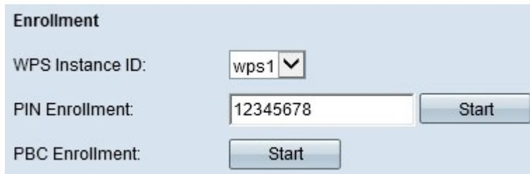
The screenshot shows a web interface titled "Enrollment". It contains three rows of controls: "WPS Instance ID:" with a dropdown menu showing "wps1"; "PIN Enrollment:" with a text input field containing "12345678" and a "Start" button; and "PBC Enrollment:" with a "Start" button.
