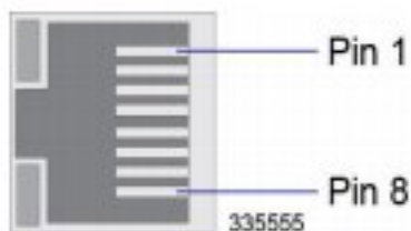
Figure 31. SPIO Ethernet RJ-45 Interface
