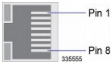
Figure 31. SPIO Ethernet RJ-45 Interface
