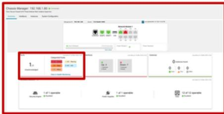
Live faults on the device are represented. The number indicates presence of fault and fault categories are listed on right side of the tile. Hover over the unacknowledged faults to show a tooltip that lists the faults.
