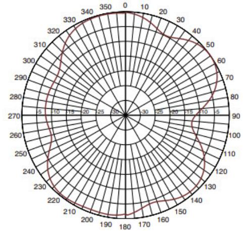
Azimuth Pattern at 2.2 GHz
