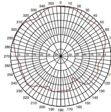
Elevation Pattern at 850 MHz
