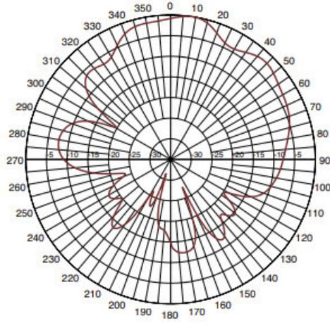
Phi-90 Azimuth Pattern at 3.6 GHz
