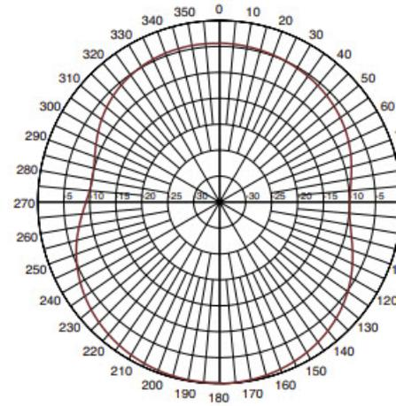
THETA-90 Azimuth Pattern at 850 MHz
