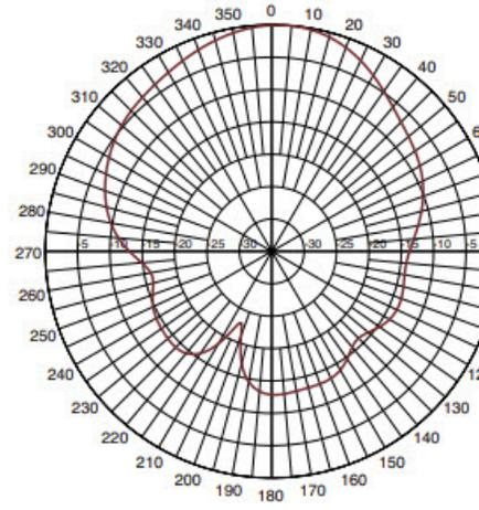
Phi-90 Azimuth Pattern at 850 MHz
