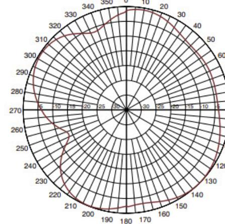
THETA-90 Azimuth Pattern at 2.2 GHz
