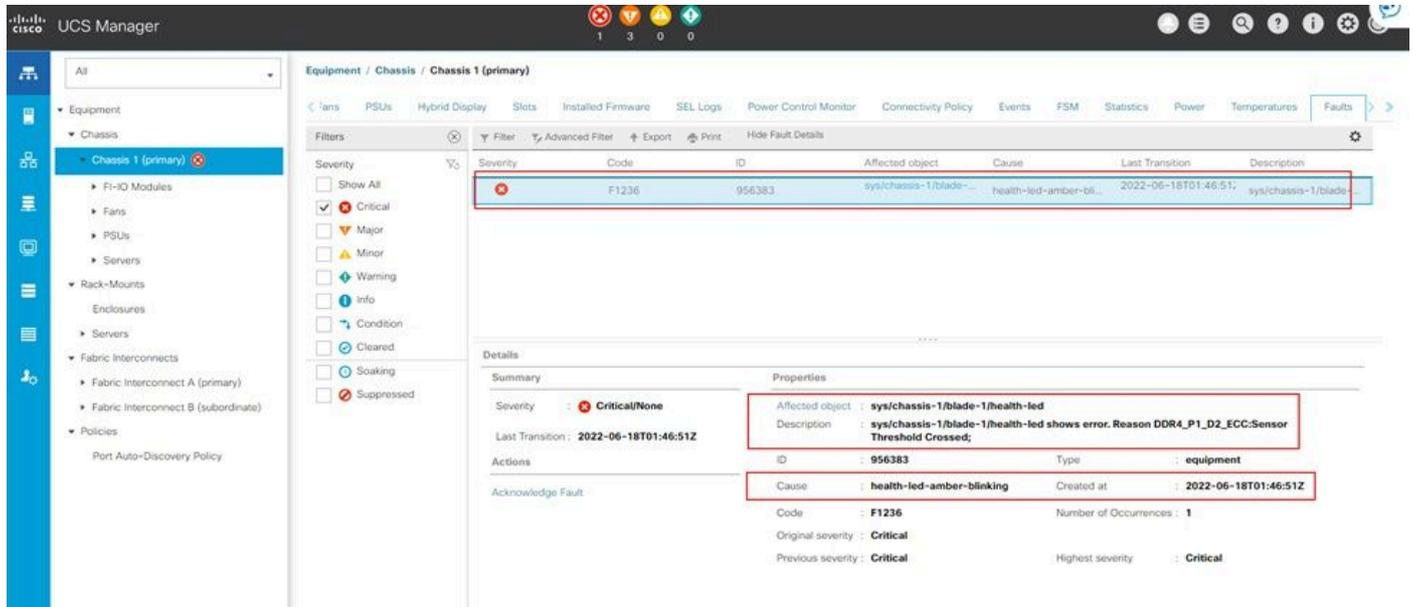
The screenshot shows the UCS Manager interface with a fault list and details. The fault list shows a fault with Code F1236, ID 956383, and Cause health-led-amber-blinking. The details section shows the affected object as sys/chassis-1/blade-1/health-led and the description as sys/chassis-1/blade-1/health-led shows error. Reason DDR4\_P1\_D2\_ECC:Sensor Threshold Crossed.
