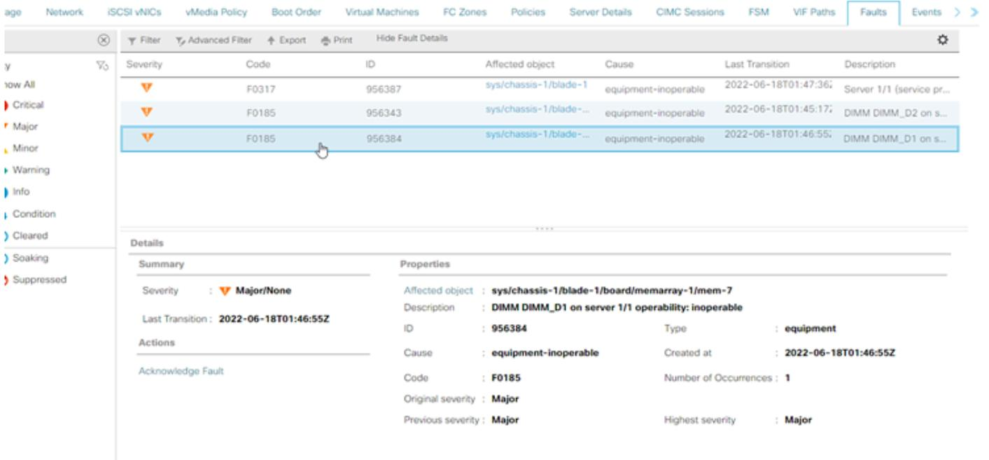
The screenshot shows the UCS Manager interface with a fault list and details. The fault list shows a fault with Code F0185, ID 956384, and Cause equipment-inoperable. The details section shows the affected object as sys/chassis-1/blade-1/board/memarray-1/mem-7 and the description as DIMM DIMM\_D1 on server 1/1 operability: inoperable.
