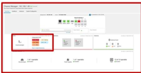
Live faults on the device are represented. The number indicates presence of fault and fault categories are listed on right side of the tile. Hover over the unacknowledged faults to show a tooltip that lists the faults.
