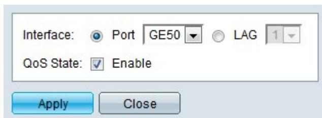
The screenshot shows the 'Modifica impostazioni interfaccia QoS' dialog box. It has two radio buttons for 'Interface': 'Port' (selected) and 'LAG'. The 'Port' radio button is selected, and the dropdown menu shows 'GE50'. The 'LAG' radio button is unselected, and the dropdown menu shows '1'. The 'QoS State' is checked and set to 'Enable'. There are 'Apply' and 'Close' buttons at the bottom.
