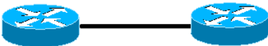
Figura 6 - Router collegati back-to-back
