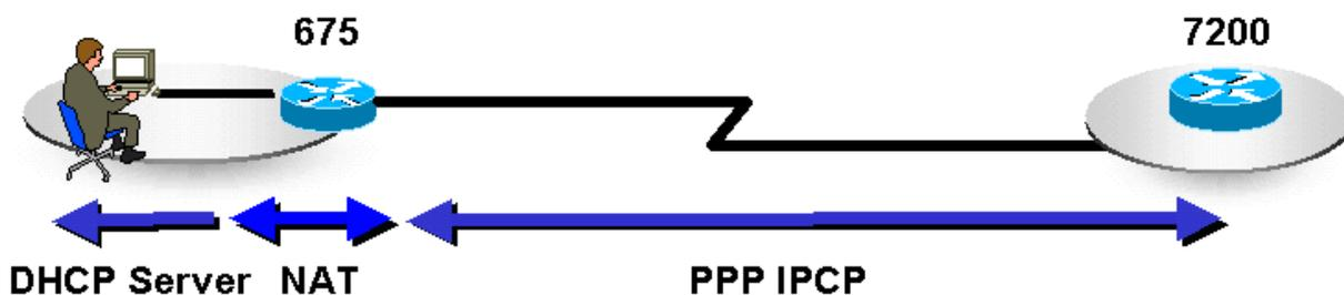
The CPE configuration in this architecture depends on NSP or the Corporate Gateway, which may terminate the PPP sessions from the subscriber. When the CPE is configured, it must have at least one set of VPI/VCI, and a username and password should be defined.
