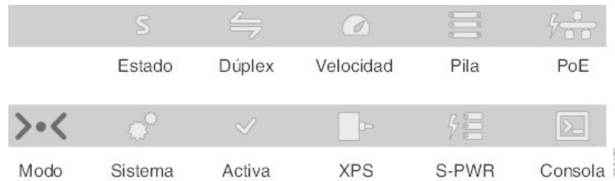
Figura 7: LED del panel frontal del switch
