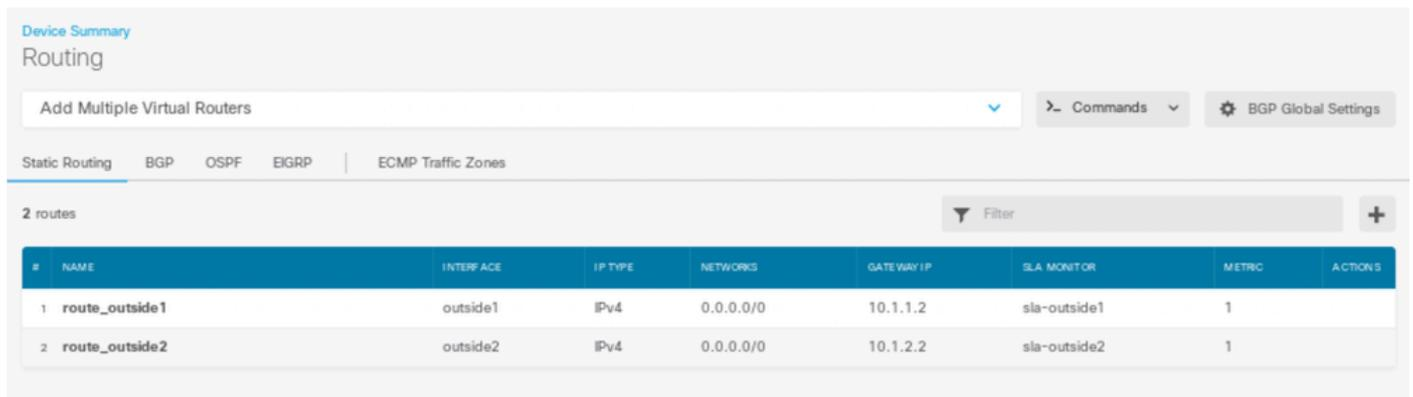
The screenshot shows the 'Routing' configuration page in Cisco FTD. It features a navigation menu with 'Static Routing', 'BGP', 'OSPF', 'EIGRP', and 'ECMP Traffic Zones'. The 'Static Routing' tab is active, displaying a table with 2 routes. The table has columns for #, NAME, INTERFACE, IP TYPE, NETWORKS, GATEWAY IP, SLA MONITOR, METRIC, and ACTIONS.
