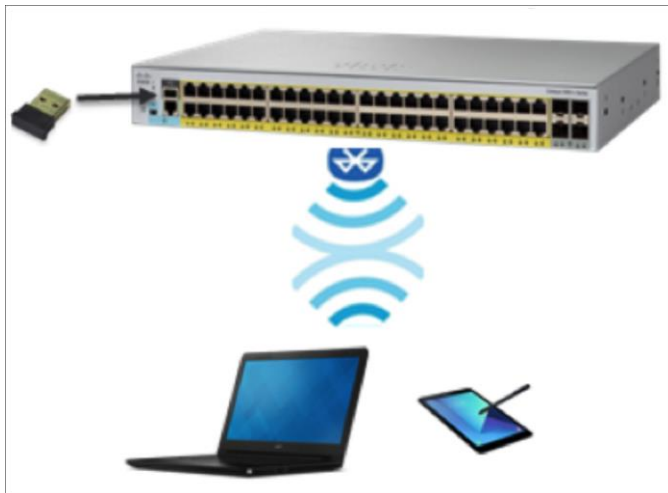
Figure 2. Over-the-air switch access using Bluetooth
