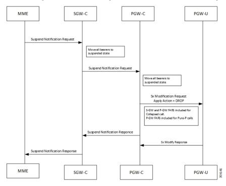
On receiving a Suspend Notification message, the PGW-C requests the PGW-U to discard packets received for the suspended PDN connection by setting the DROP flag in the Apply Action IE of the FARs of the corresponding PFCP session.
