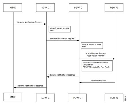
On receiving the request to resume the PDN connection, the PGW-C re-allows the PGW-U to forward the packets for the PDN connection by:
