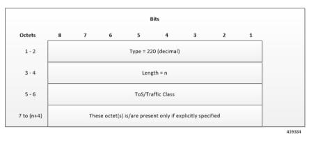
The encoding for ToS/Traffic Class takes place in the form of two octets as an OctetString. The first octet contains the DSCP value in the IPv4 ToS or the IPv6 Traffic Class field and the second octet contains the ToS/Traffic Class mask field, which is set to 0xFC.
