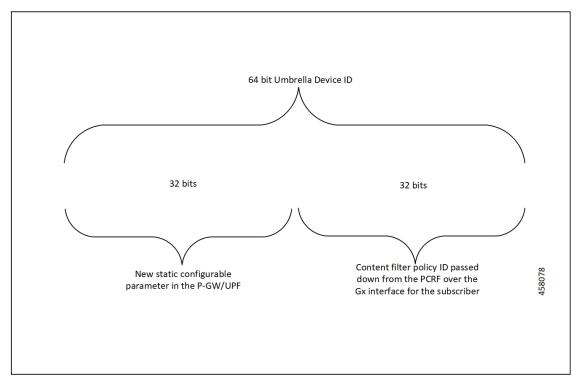
The Device ID number in the EDNS0 record allows the Umbrella DNS system to apply a custom set of domain filters for the EDNS0 queries.
