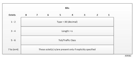
The encoding for Type-of-Service (ToS) or Traffic Class takes place in the form of two octets as an OctetString. The first octet contains the DSCP value in the IPv4 Type-of-Service or the IPv6 Traffic-Class field and the second octet contains the ToS/Traffic Class mask field, which is set to 0*xFC*.
