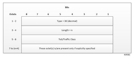
The encoding for Type-of-Service (ToS) or Traffic Class takes place in the form of two octets as an OctetString. The first octet contains the DSCP value in the IPv4 Type-of-Service or the IPv6 Traffic-Class field and the second octet contains the ToS/Traffic Class mask field, which is set to 0xFC.
