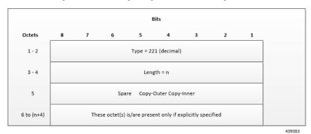
The Copy-Inner and Copy-Outer flags are present in bit-0 and bit-1 of octet 5. Copy-Outer flag is not used for downlink packets because there is no outer header present in packets coming from ISP. If a Copy-Inner flag is present, then the UPF uses DSCP value from the inner packet to mark the transport-level IP header.
