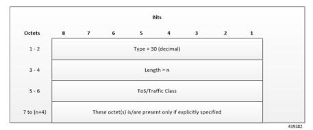
The encoding for Type-of-Service (ToS) or Traffic Class takes place in the form of two octets as an OctetString. The first octet contains the DSCP value in the IPv4 Type-of-Service or the IPv6 Traffic-Class field and the second octet contains the ToS/Traffic Class mask field, which is set to 0xFC.
