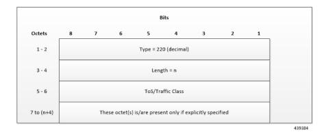
The encoding for ToS/Traffic Class takes place in the form of two octets as an OctetString. The first octet contains the DSCP value in the IPv4 ToS or the IPv6 Traffic Class field and the second octet contains the ToS/Traffic Class mask field, which is set to 0xFC.
