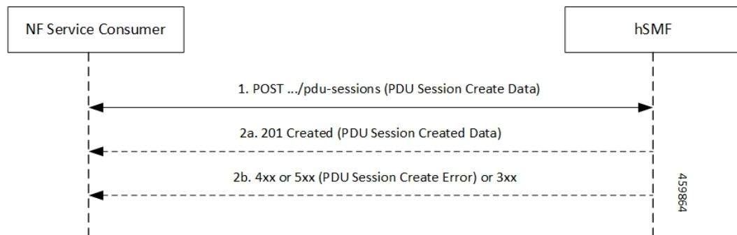
Figure 6: Create Service Operation on hSMF Call Flow
