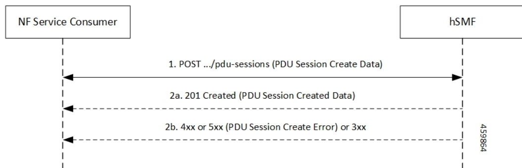
Figure 109: Create Service Operation on hSMF Call Flow
