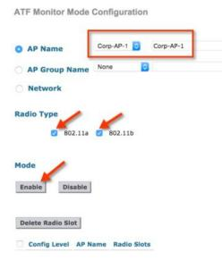
Once configuration is done it displays the config level, AP name and radio slots (Slot 0 is 802.11b Radio and Slot 1 is 802.11a Radio) on which monitoring is enabled.
