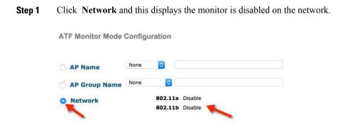
Step 2 Choose the Radio Type by checking the 802.11a or 802.11b or both radio boxes then click Enable under the Mode option
