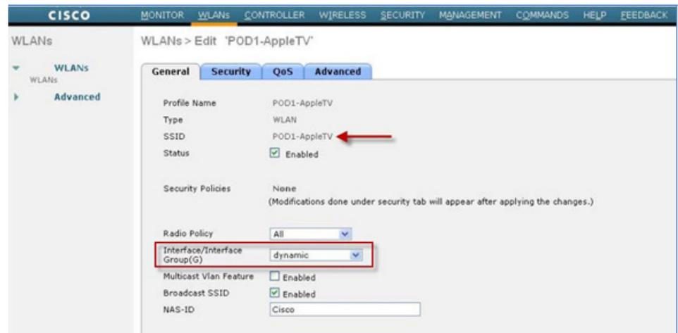
6. Connect the Apple TV to the service set identifier (SSID) created for device services, and connect the Bonjour client (iPad/iPhone) to the SSID for clients.
