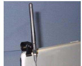
**Step 3** Install the antenna's cable into the external jack on the Sensor card using the cable plug (MMCX male connector).
